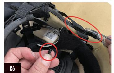
PAC FIRE RECOMMENDS USING NEW RIVETS & PIVOT PLATES WHEN REPLACING RESCUE EYE PROTECTOR.
